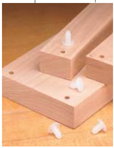
▲ Plastic "stem bumper glides" are added to the front of all the lower drawer supports (and top, back corners of the drawers) so they slide in and out of the case smoothly.
