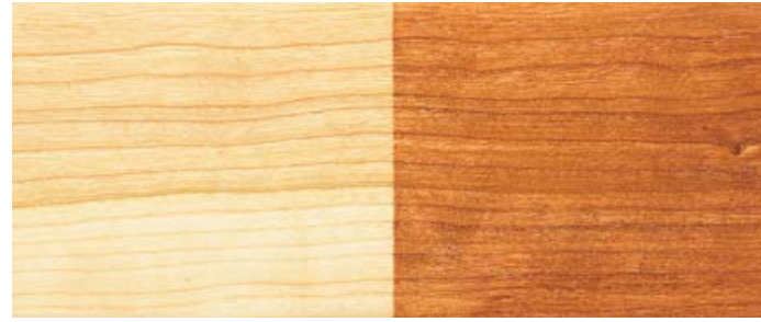
▲ The light sapwood in this board won't darken with age. But a single coat of cherry stain can hide it.
